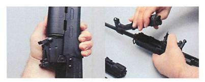
To install the gas tube shroud rail use vice grips or table vice to grab the flat spots on the rear if the gas tube. Firmly rotate the shroud 180 degrees and slide it out of the bottom. Make sure to reinstall the retaining spring on the new shroud prior to installing onto the gas tube. Reverse the process to install.
