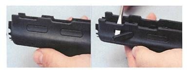
Slide the hex nut in the groove inside the handguard and hold it with your finger, insert the rail in the appropriate slot and use the provided Allen screws to hold the rail in place. Do not over tighten the screws thread locker may be used to ensure that no hardware will loosen under use.
