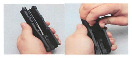
Use a small screwdriver or punch to poke through the mounting holes on the inside of the handguard.
