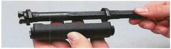
To install the rails on the lower handguard flip the lever on the retainer and slide the retainer forward.
