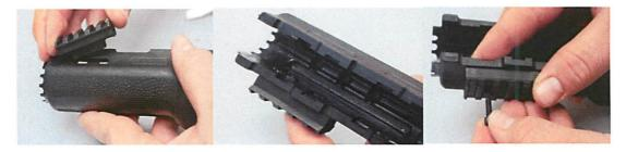
Reinstall the heat shield and reverse the disassembly procedure to assemble the firearm. Verify fit and function check the firearm.
